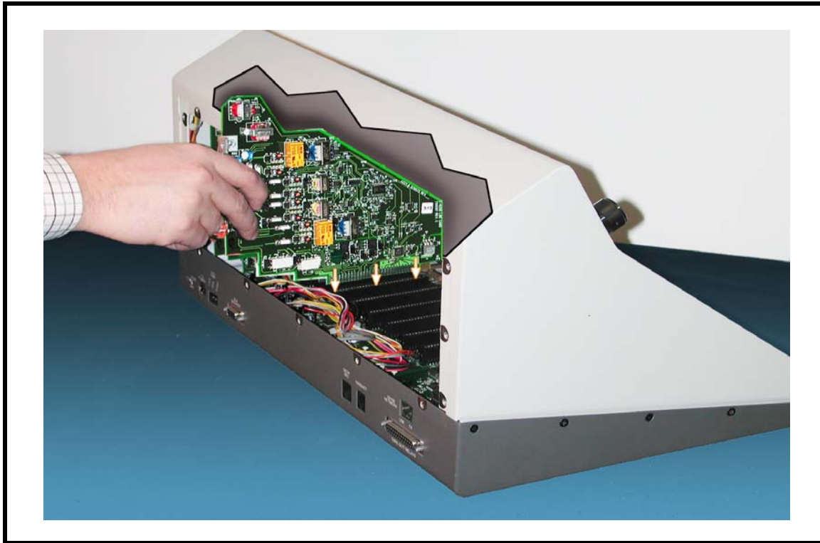
FIGURE 13. Line Card Installation—Cutaway View
