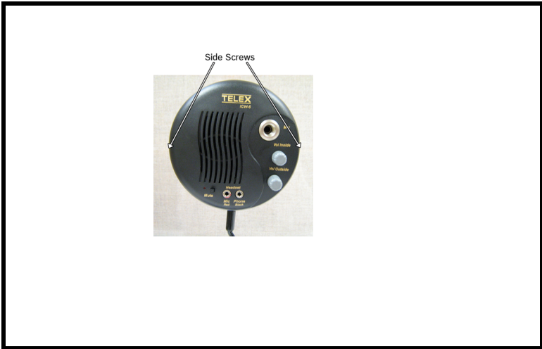
FIGURE 8. Side Screws Holding the Back Plate to the Operator Unit
