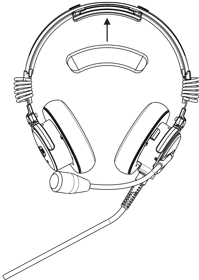
Figure 6.4: Installing New Headband Pad
