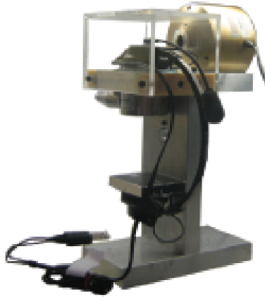
Figure 6.6: Custom ANR test fixture with headset
