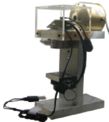
FIGURE 9. Custom ANR Test Fixture with Headset NEW PHOTO?
