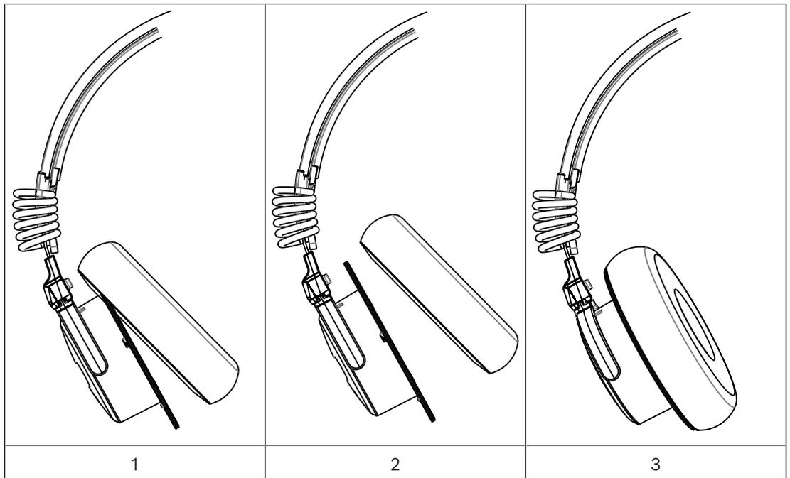
5. Verify the **replacement** is fully seated by visually inspecting around the cushion before use.
