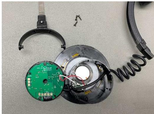
4. Using a T-5 screwdriver, remove **two screws** (as shown).
