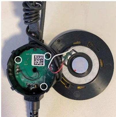
4. Remove the **housing and the yoke/glider assembly**.
