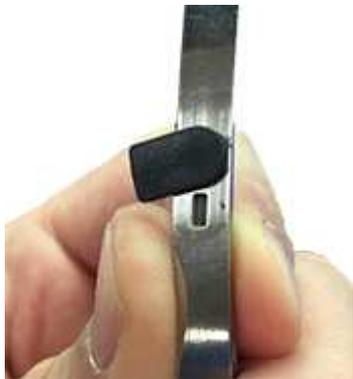
4. Click the **bottom edge of the black plastic spacer** into the retaining hole.
