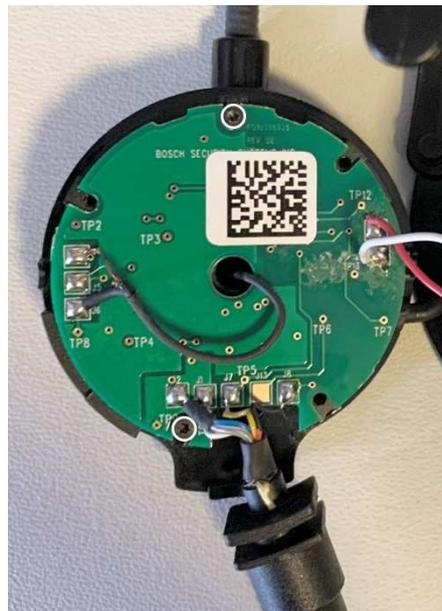
5. Solder the **boom mic wires to the PCBA**.
