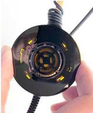
3. Using a T-5 screwdriver, remove **three screws** (as shown).
