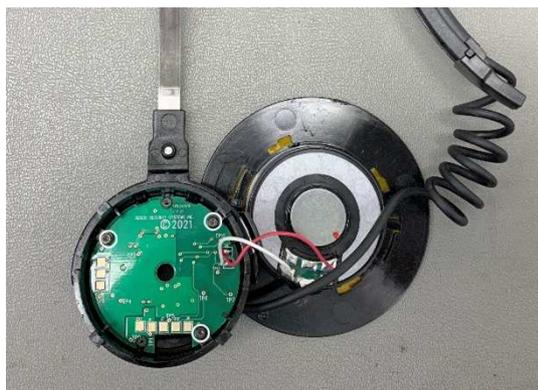
3. Remove the **housing and the yoke/glider assembly.**
