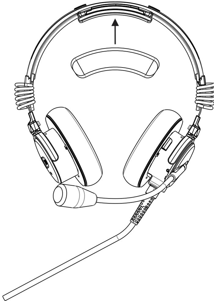
4. Firmly press **the new headband pad** into place.
