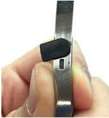
3. Slide the **yoke assembly** off of the headband.
