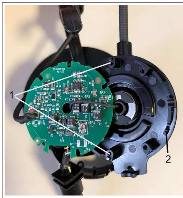
1. Alignment post for the PCBA screw
