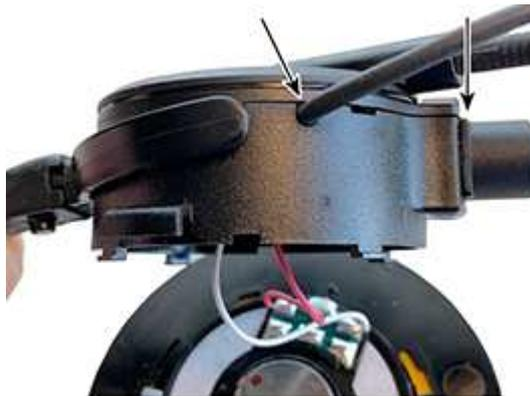
11. Using a T-5 screwdriver, replace the **three screws** (as shown) to attach the yoke and housing to the PCBA.
